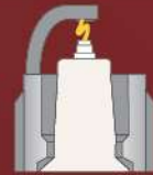
② fire moves sideways and internal short circuit discharge
