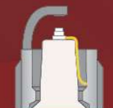
② fire moves sideways and internal short circuit discharge
