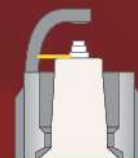
② fire moves sideways and internal short circuit discharge
